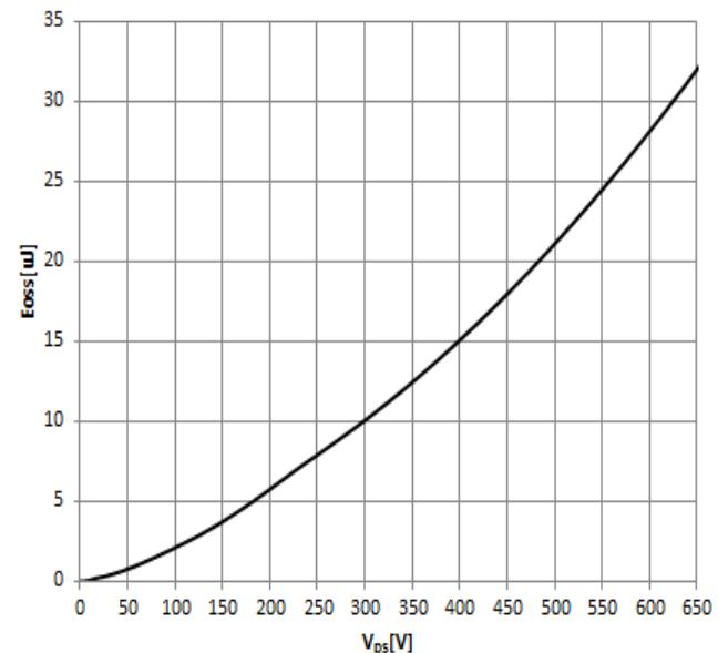
**Figure 6. Typical  $C_{oss}$  Stored Energy**
