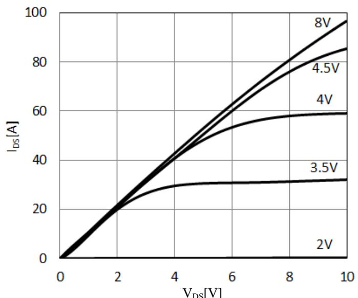
**Figure 2. Typical Output Characteristics  $T_J=150^\circ\text{C}$**
