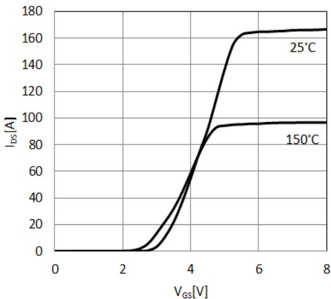
**Figure 3. Typical Transfer Characteristics**
