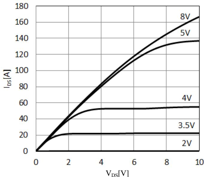
**Figure 1. Typical Output Characteristics  $T_C=25^\circ\text{C}$**
