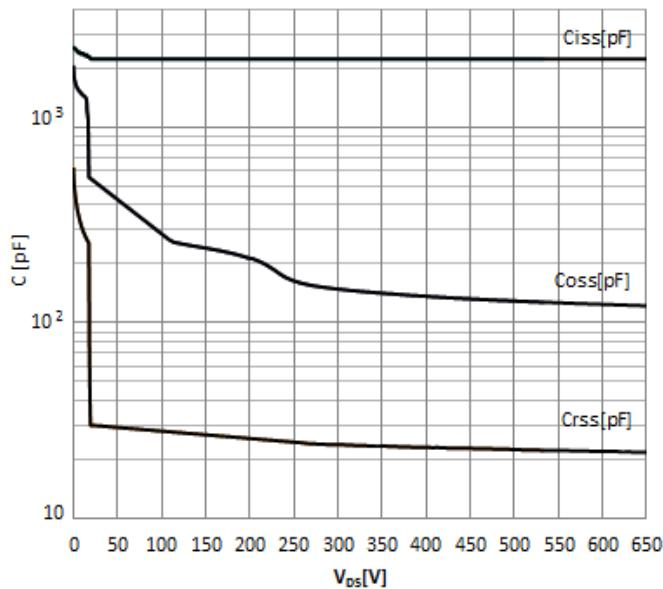
**Figure 5. Typical Capacitance**
